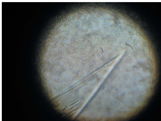
Figure 2 Morphology of Rv3002c crystals. The approximate dimensions of Rv3002c crystals of diffraction quality grown over a period of 3–4 d were 10 \times 50 \times 200 \mu\text{m} .
